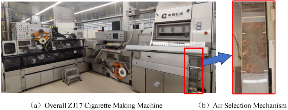
Figure 1. Diagram of the ZJ17 Cigarette Making Machine
